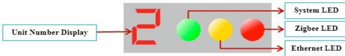
Figure 9-1. LED Display Panel on top of Maxx-1100 unit. These LEDs indicate status of different modules of the unit.
